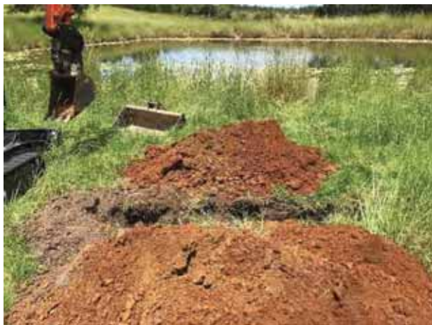
Excavated material from TP9. 0.7m of topsoil was encountered and overlies very stiff residual Silty CLAY
