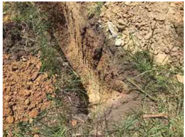
TP4 which was excavated in the west of the northern portion of the site and encountered yellow-brown residual Silty CLAY that overlies weathered Phyllite
