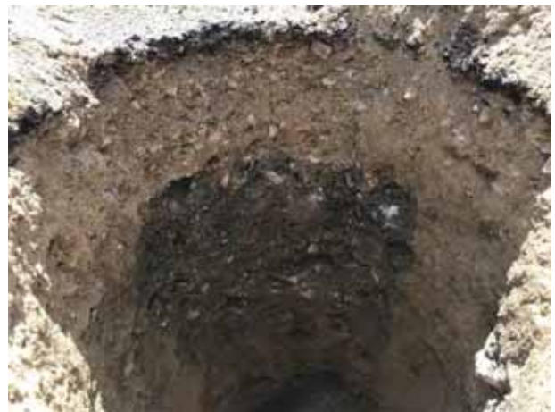
BH2 which was drilled within Red Ash Road and encountered 0.16m of pavement gravel over gravel fill to 1m, overlying highly weathered phyllite
